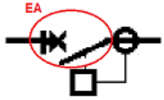
Effektafbryder (Circuit breaker)
